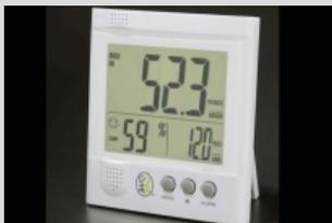
Smart meters offer the dwelling's occupants a real-time view of their energy usage (electricity, energy associated with heat and hot water, and sometimes also water use), and so can help to eliminate unnecessary use, and reduce running costs, resource use and CO<sub>2</sub> emissions. Some displays can also provide local public transport information.
